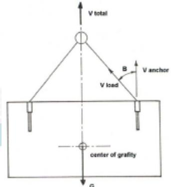
The adapted load ( $V_l$ ) = increase factor (z) x the total load/anchor ( $V_a$ )
