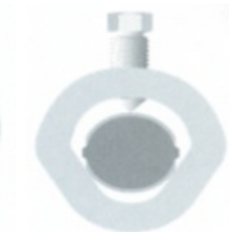
Couplers for rebars size 12mm to 32mm
